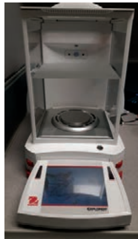
New Analytical Balance used to calibrate hydrometers for FBO ATA 103 compliance.
