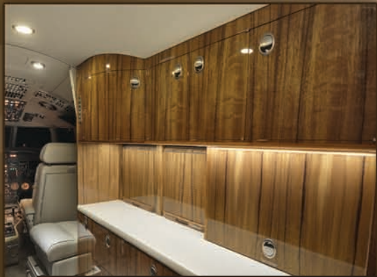
Modified galley with new counter and oval latches to update the design.
