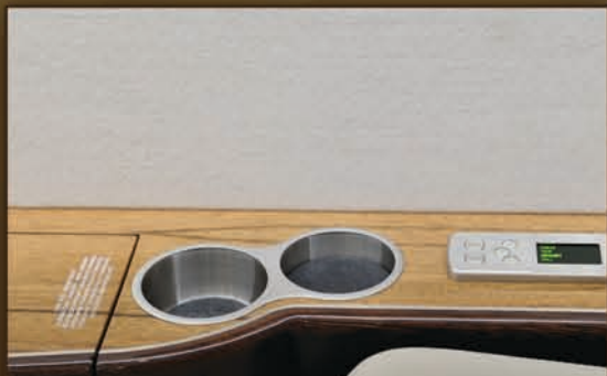
Duncan designed figure eight cupholders and new passenger controls including a custom bracket to angle the control screen for improved passenger viewing.
