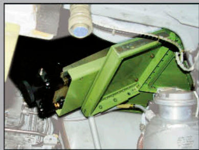
After the modification, access to the avionics boxes is through the nose wheel bay. These images show one of the shelves tilted down for box removal. The left and right images are taken from the wheel bay. The center image is taken from the opposite avionics bay.
