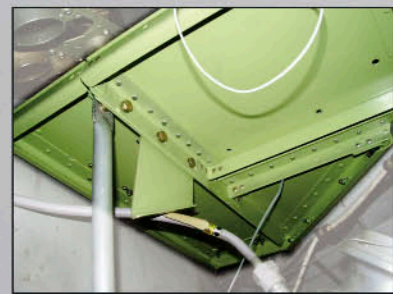
The modification of the shelf consisted of being split, installing a down-swing hinge and adding strong anchor bolts.
